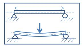
A simply supported beam is a member that only supports the vertical loads at each end. No horizontal force or moment (torque) is present.
